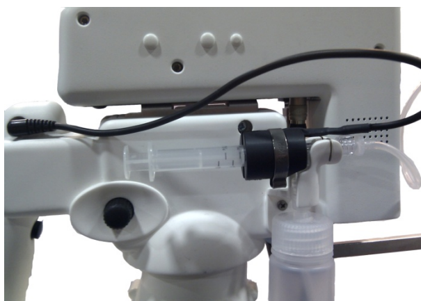
Figure 10: The acetic acid application mechanism
